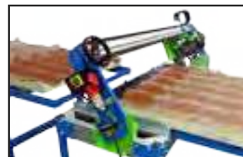
Special model, adapted for cutting polyurethane insulating panels.
