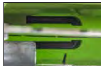
Water cooling fork, reaching both blade sides.
