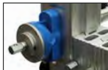
Speed reducer gearbox: High - Low speed.
