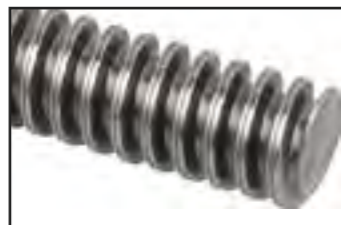
Cutting depth operated by trapezoidal thread shaft.
