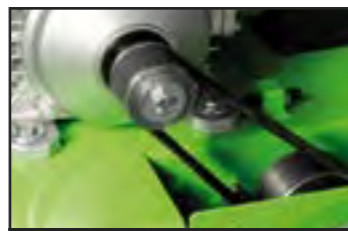
Poly-V belt transmission improves grip and reduces maintenance (BALI 500 MK).
