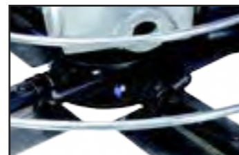
Blade holders include a lubricator nipple for an easier maintenance.
