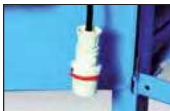
Internally mounted power socket to reduce wear and tear.
